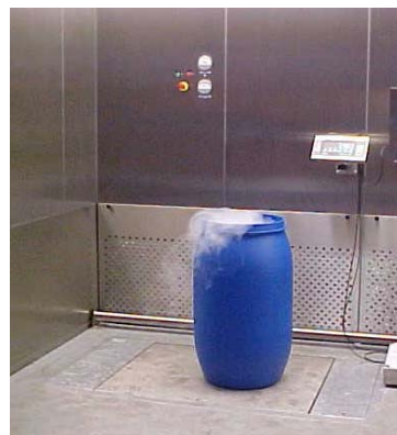
Smoke test at FAT to confirm air circulation and operator protection
