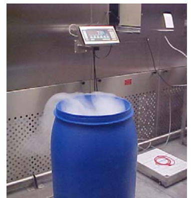
Smoke test at FAT to confirm air circulation and operator protection
