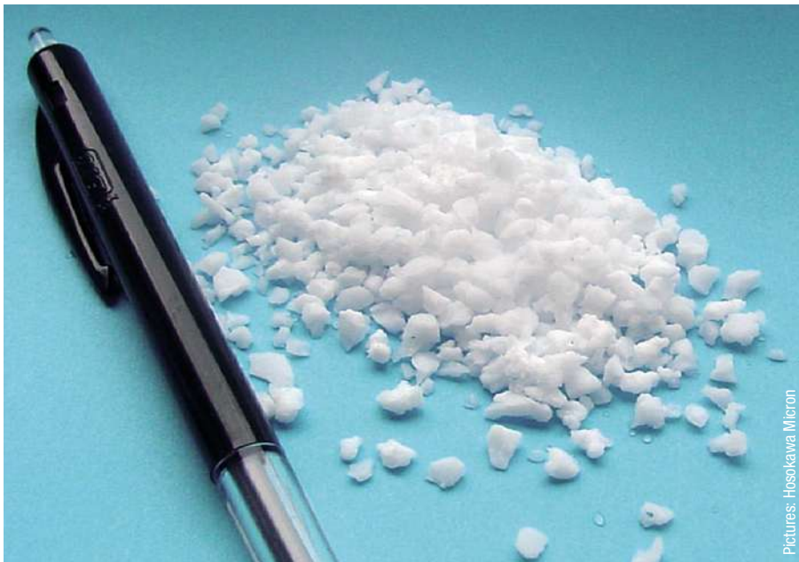
Frozen granular material as produced in the freezing step with Active Freeze Drying
