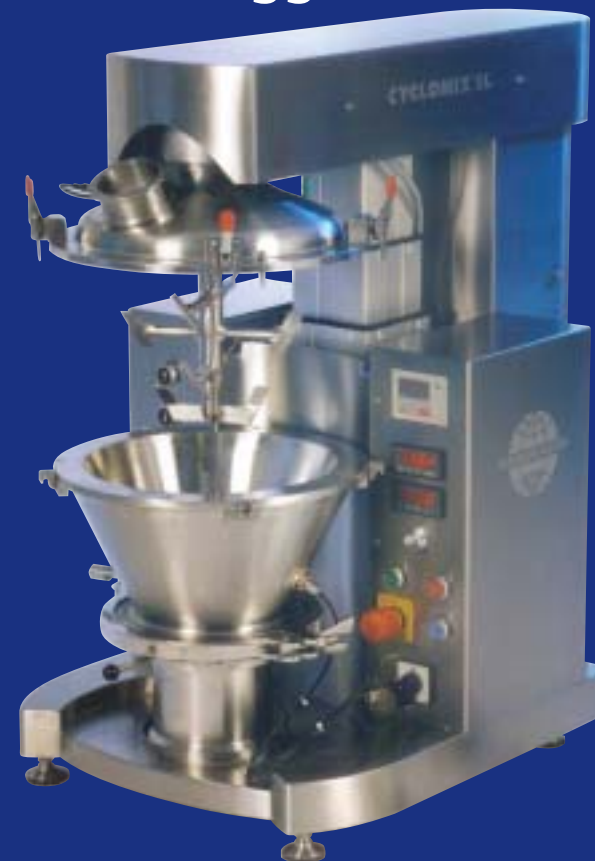
Figure 1. 5-L Cyclomix high shear mixer/agglomerator, manufactured by Hosokawa Micron B.V.
